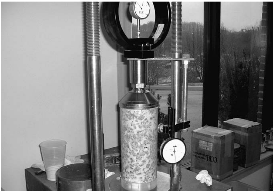
Figure 2. Grout Sample Prior to Unconfined Compression Testing
