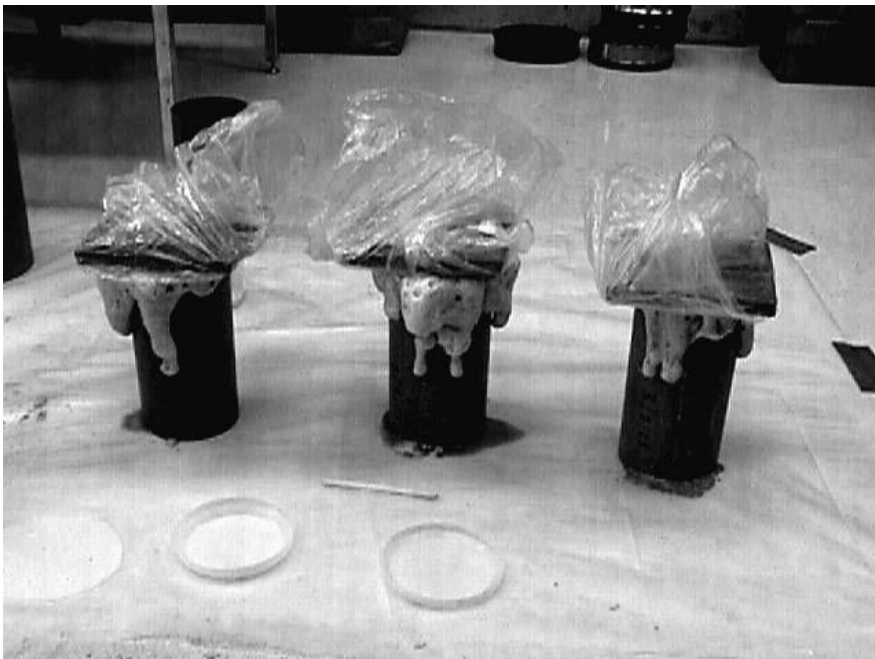
Figure 1. Polyurethane Sample Formation. Note grout foaming through drainage holes at the top and bottom.
